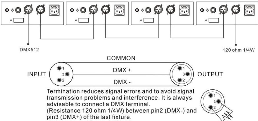
1. If you using a controller with 5 pins DMX output, you need to use a 5 to 3 pin adapter-cable.
